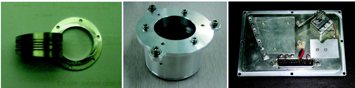
Figure 10. A spring unit (left), a filter module assembly (middle) and a sensor module (right).
