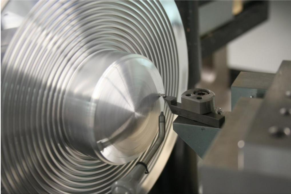
Figure 3.3 Machining image of the primary mirror. Off-axis primary mirror is manufactured by Freeform 700A. The nozzle which is under the diamond bite ejects mist (oil + air) to eliminate chips easily.
