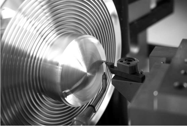
Fig. 5. — Machining of the primary mirror using Freeform 700A. The nozzle seen under the diamond bite ejects mist (oil and air) to eliminate chips easily.
