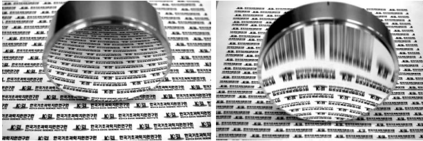
Fig. 6. — Fabricated primary mirror (left) and secondary mirror (right) of the off-axis telescope.
