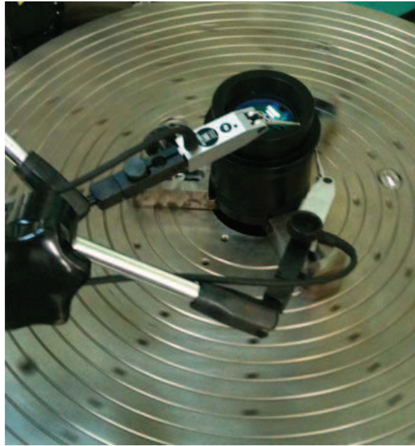
Fig. 7. — Alignment setup for the lens module of the focal reducer. Initial placement of the lens barrel is being measured by the probes on the testing plate.
