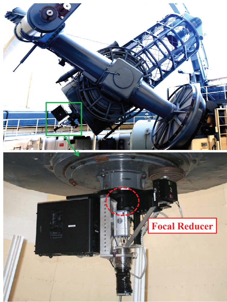
Fig. 9. — CQUEAN attached to the 2.1 m Otto Struve telescope. Science CCD camera is the silver box in the center, and guide CCD camera is the small black box in the upper right part of the system. The big black box in the left is the control PC. The motor below the science CCD camera moves the arm to rotate guide CCD camera (Kim et al. 2011). The location of the focal reducer is indicated in the bottom panel.
