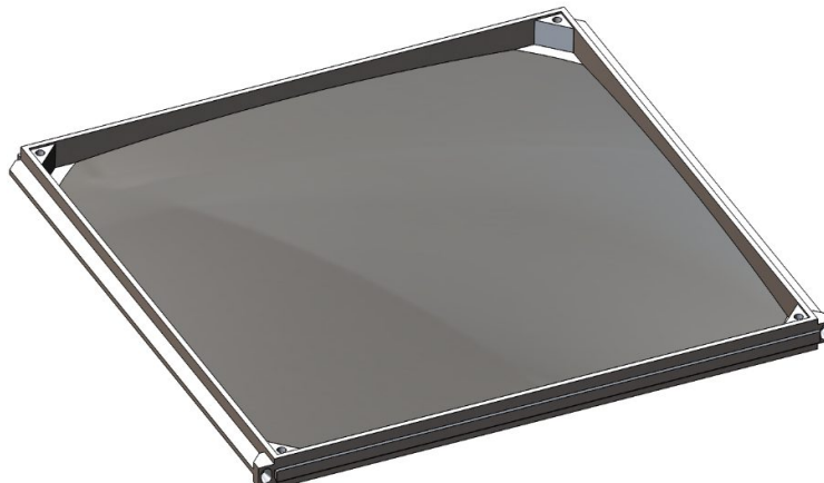
Figure 7. Concept of the GMACS slit mask in its cartridge.
