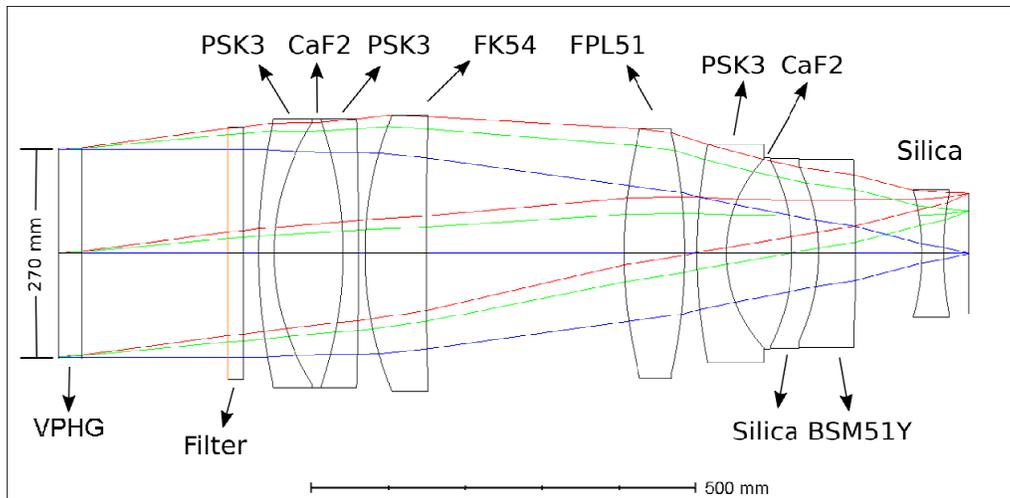
Figure 3. Blue camera in imaging mode
