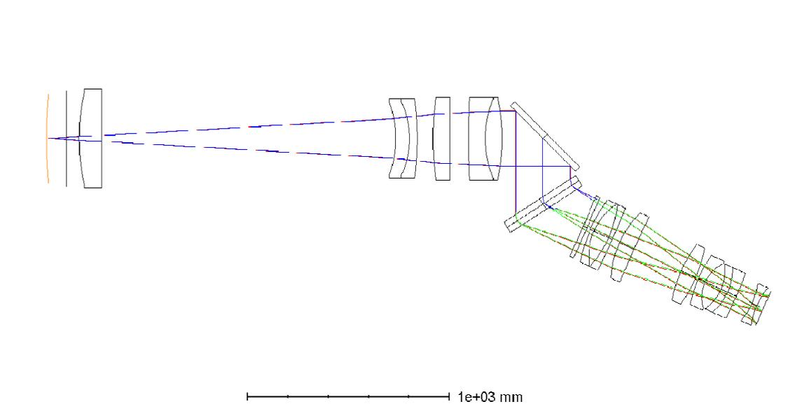
Figure 13. High resolution spectrograph layout for blue arm
