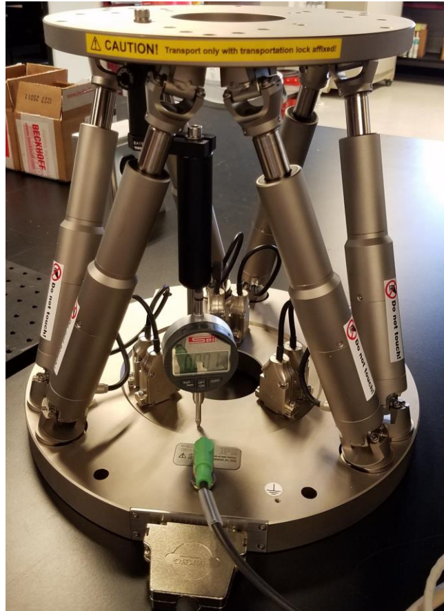
Figure 3. Physik Instrumente H-840.D2 hexapod
