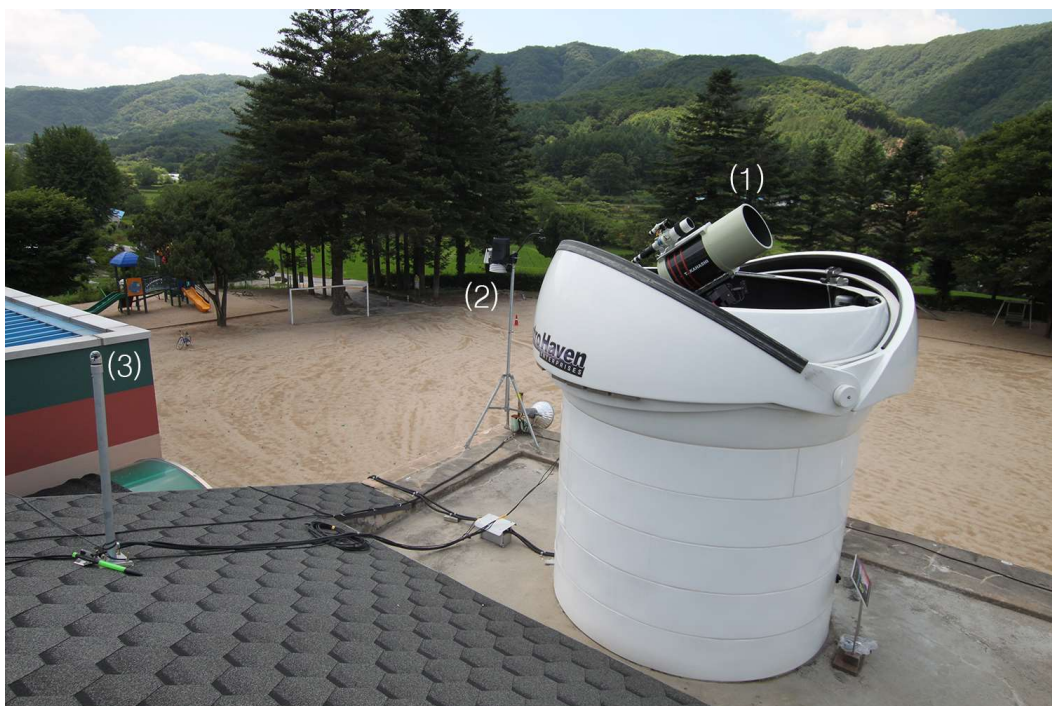
Figure 2. The exterior appearance of MURO. (1) 2.1m fiberglass clamshell dome, (2) weather cast, (3) all sky camera.
